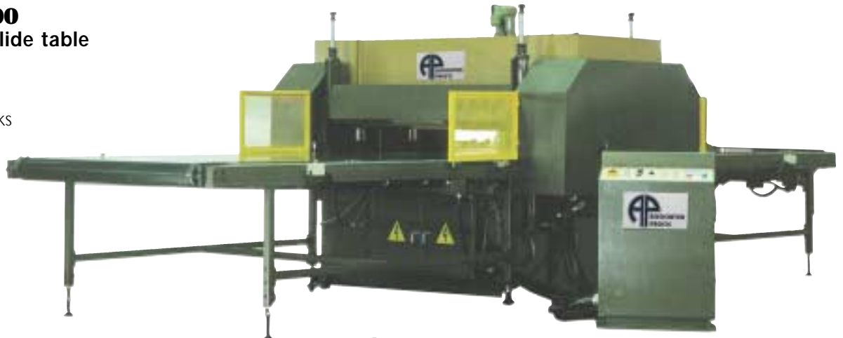
USA - FH 3563-150 Cutting against poly pad and pad shifter
